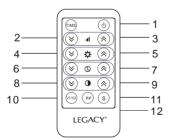
1.Power On/Off 2.Volume -3.Volume + 4.Brightness -5.Brightness + 6.Colour-7.Colour + 8.Contrast-9.Contrast + 10.V1/V2 switch 11.Store 12.Display mode
